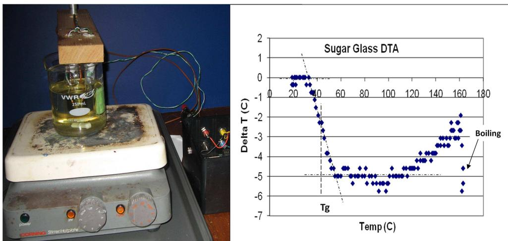
Figure 13. Photograph of the DTA apparatus with Basic Stamp microprocessor for temperature measurement and data logging. A sample DTA scan for the candy glass is shown on the right, with midpoint  $T_g$  indicated.
