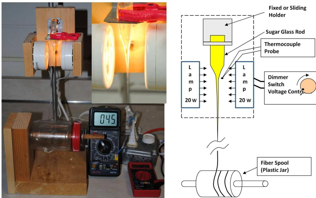
Figure 5. Photograph of our home-made fiber drawing tower for candy glass using two halogen lamps for the “furnace”. A sketch of the components for measurement and control is shown on the right.
