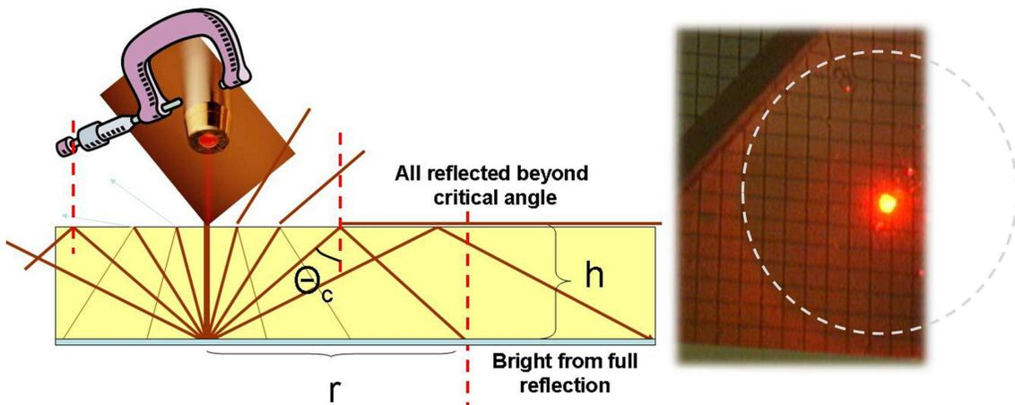
Figure 3. Basic concept of Pfund's method for measuring the refractive index of a transparent plate. Photo on right show darker region in the center of sugar glass slab.
