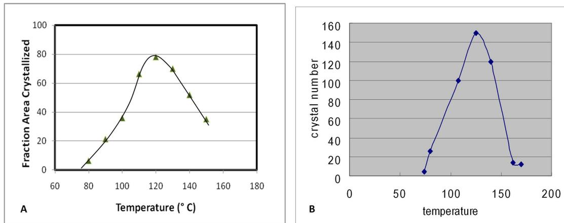
Figure 11. Examples of data measured in two different student experiments. Crystal growth rate vs. temperature in A) done by a college level REU student using Image J to extract the area from photos while B) performed by a high school student using the simple method of estimating the number of “crystal spots”. Note the distinct maximum near 120° C for both approaches.
